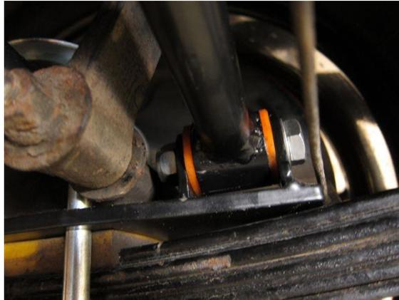
16. Check everything is in order (i.e. adequate clearance of the petrol tank); if so then tighten up the rod locking nut and the nut and bolt on the Axle Plate.
