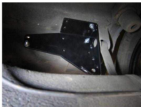
7. Ensure the bracket remains snugly fitted against the axle strap bracket and surfaces A + B before drilling the remaining holes.
