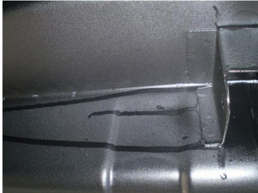
5. Offer up the body mounting bracket against faces A & B and hard up against the axle strap bracket. When happy that the bracket is a close snug fit to the surfaces use the bracket as a template to mark two well spaced holes on each surface to locate the bracket. (See Image below)
