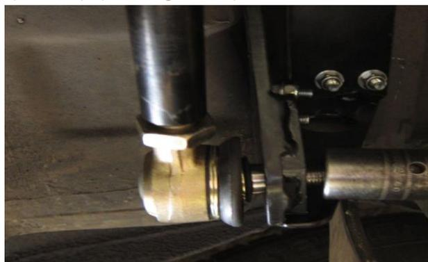
15. By screwing the ball joint into the rod attach the bush end of the rod to the axle bracket, do not tighten just yet. The rod length should be neutral and not required to be pulled or pushed to engage the Axle Bracket/Bush bolt cleanly. (See Image below)
