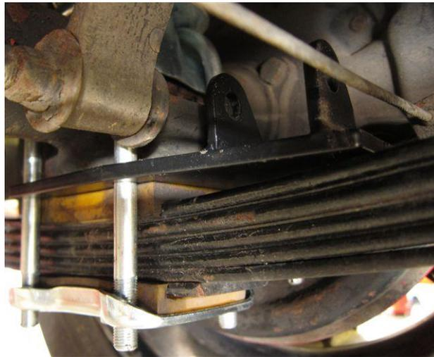
13. Assemble and evenly tighten the U bolt nuts. (There is no torque specified in the workshop manual for these but we'd suggest 25 to 30 ft/lbs)
