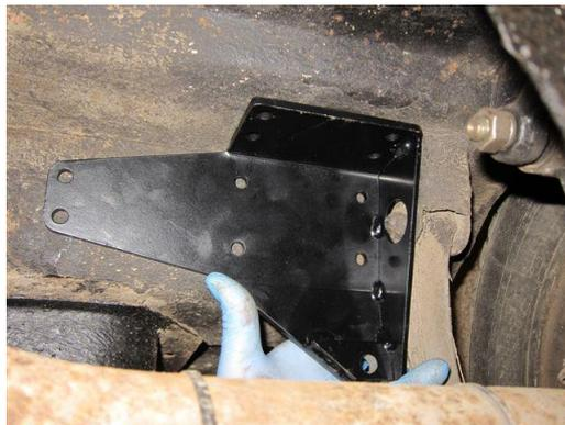
6. Pilot drill the holes, re-drill to 8mm and then pass the bolts with large washers through the boot floor and secure the bracket using the plain nuts. (See Images below)
